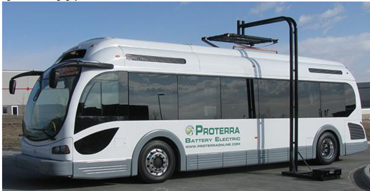
Figure 1: Fast Charging System
