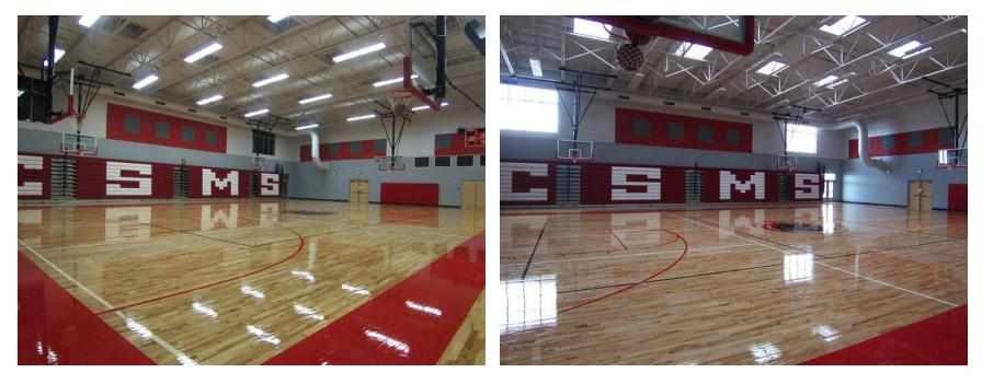
By night: 500 lux, 0.65 w/sf, 5 kwh/hr of lighting load, .65 w/sf of cooling load
