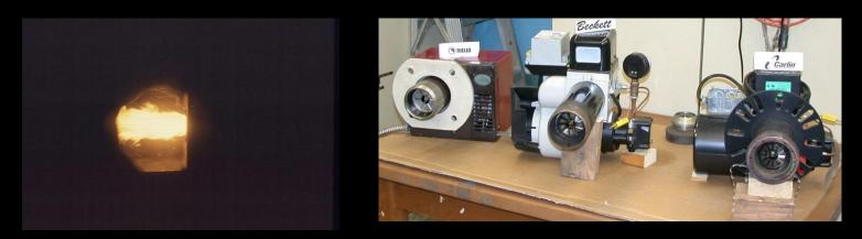
With oil burners having a lower limit between 50k Btu and 70k Btu, the firing rate is way too high for energy demands, unless something can be done with the heat
