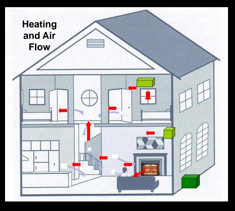
The Mini-Split can also help move the heat from the wood stove around the house, in an "unobtrusive" fashion, using its efficient fan system
