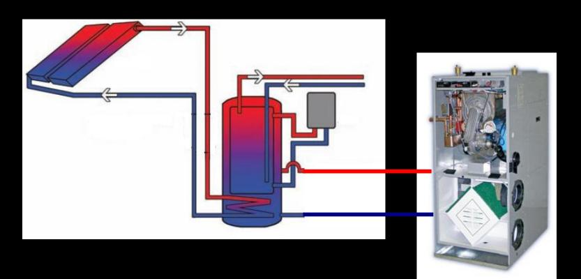
Space Heating, Water Heating, Ventilation Driven by Solar Energy & High-Modulation Gas-Fired Condensing System (possibly PV-driven)
