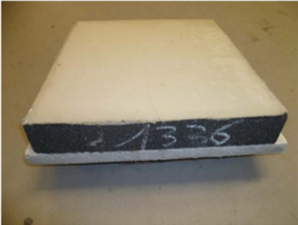
shear failure after thermal cycling
