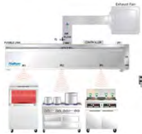
Duct Temperature Sensor & Infrared Sensors
