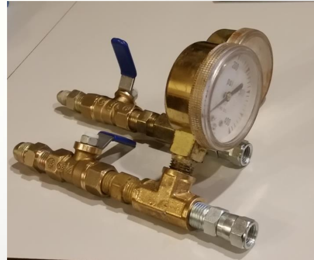
A & B pressure gauges on valve sets
