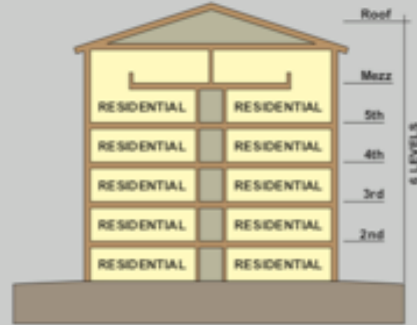
IBC Section 505: Mezzanine
